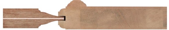
Section view of panel and stile of a Portobello door. Note the wider stile, thicker panel and heavier exterior molding profile.
